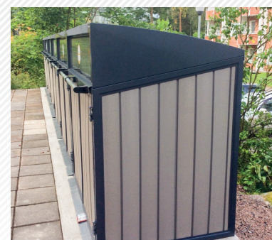
The curved roof directs the water and snow towards the back. The threshold ramp facilitates easy waste bin removal and return.
